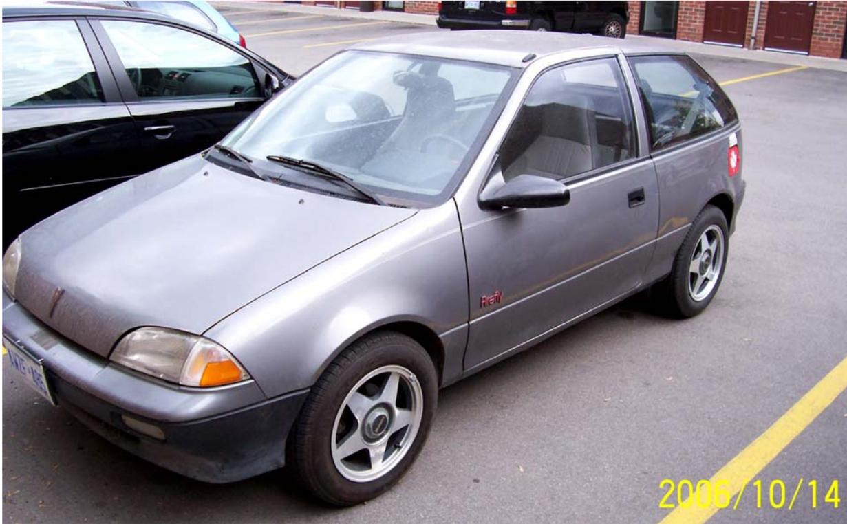
This car is a conversion from a 1989 Pontiac Firefly, 3-Cylinder Hatchback. A Shop Teacher and a Group of High School Students originally converted it, and with it's first set of Batteries, got a range of 60 Kilometers/40 Miles.
